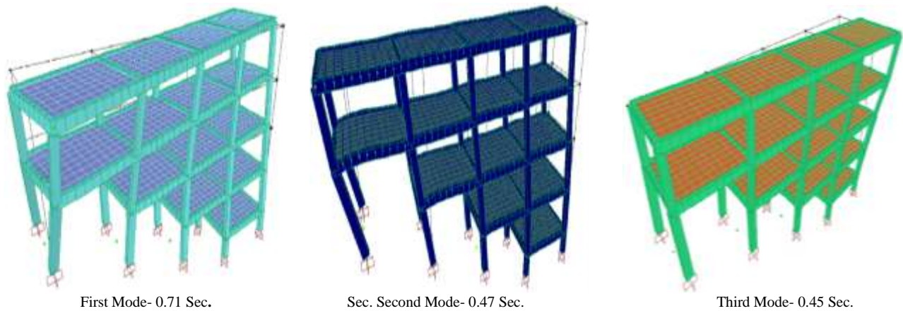
Fig.4 Fundamental mode shapes and time period
